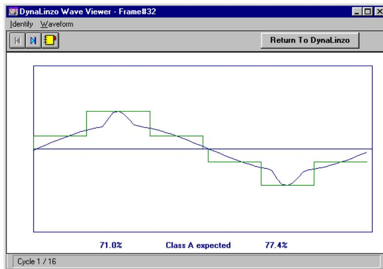
You can also view the list, which estimates an applicable class depending on the multiple waveform shapes in the frame. Select **Identify | Class** menu and then a dialogue box that includes a list of identification result will appear.
