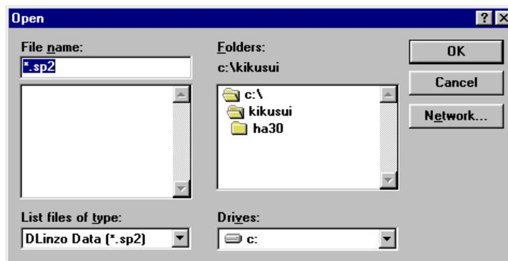
DynaLinzo has different file format and extension name between VER2.x or earlier and VER3.0 or later. (File extension of pre-VER2.x was SP1, and post-VER3.0 is SP2.) The DynaLinzo 3.0 can read old SP1 files by converting the format.
