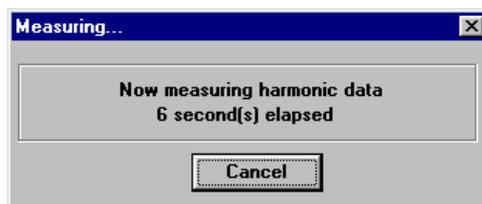
If you intend to measure with synchronisation with your device or other instrument, apply a trigger signal to the **EXT TRIG** terminal on the HA01 unit at this state. This trigger timing will reset the internal timer. However, appearance of elapsed time or remaining time will not be reset.
