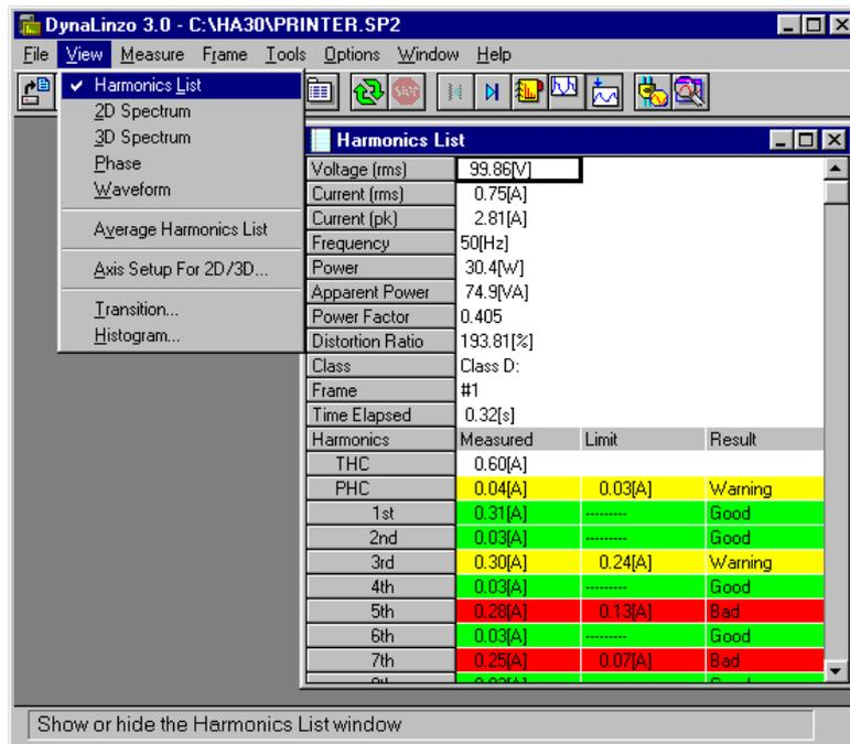
Content of the window is a list that displays harmonics data at one moment as a numeric format. Not only harmonics components, situation data such as voltage or current is also shown. This window is displayed as default and you can show or hide it operating **View | Harmonics List** menu. The list is shown as a spread sheet style and each cell of harmonics components is represented in colour so that you can distinguish the results of harmonics judgement as described below.
