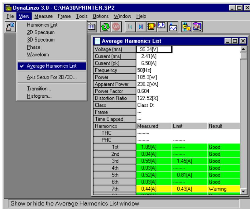
Content of the window is a list that displays average harmonics data over the entire test period as a numeric format. Not only harmonics components, situation data such as voltage or current is also shown. This window is not displayed as default and you can show or hide it operating **View | Average Harmonics List** menu. The colour separation in the result view is the same as (non-average) Harmonics List.
