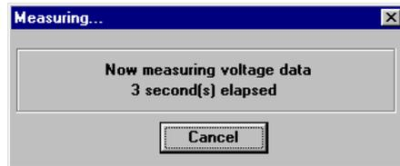
After the measurement has been done, all of the data will be automatically downloaded and will be displayed on the VF-Analyzer screen.
