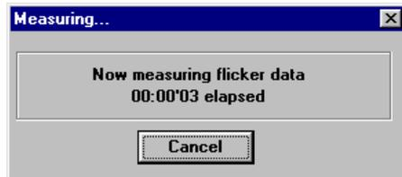
Unlike DynaLinzo and VF-Analyzer applications, there is no functionality of external trigger on the Flicker Analyzer. Applying a trigger signal onto the **EXT TRIG** terminal causes not only meaningless operation, but also breaks measurement session itself. So you should not apply any external trigger signals during flicker measurement.
