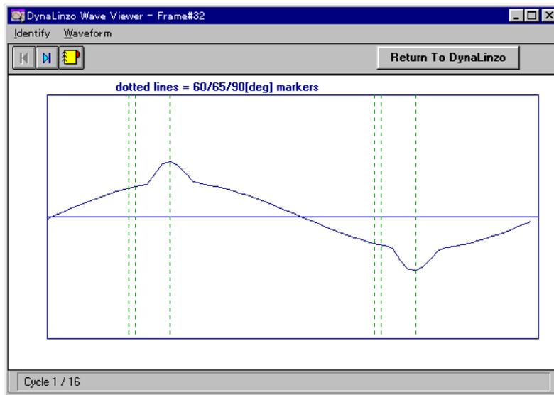
These gridlines shows 60/65/90/240/245/270[deg] locations based on the voltage phase. Evaluate the current phase by following to the requirements of the IEC std or Japan Guideline. Selecting **Identify | Phase** menu also displays phase angles and current values for each data point, and utilize these data for identification work. In the display, the data coloured in red means the positive peak, and the data coloured in blue means the negative peak.
