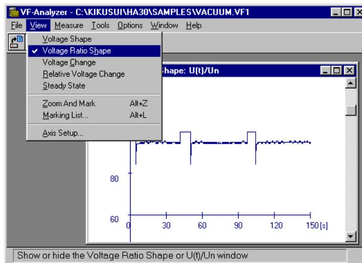
This window represents transition of voltage ratio (rms voltage / nominal voltage) values for both positive and negative. Other than graphic contents are exactly the same as Voltage Shape  $U(t)$  window.
