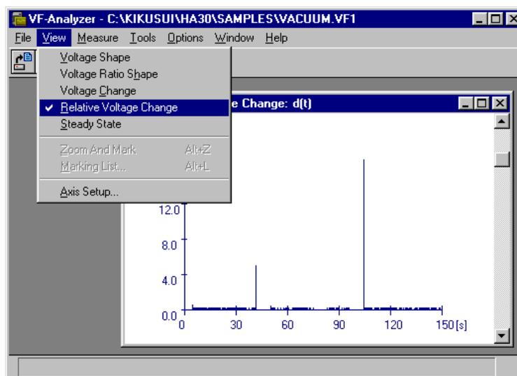
This window represents relative values of above mentioned **Voltage Change  $\Delta U(t)$**  graph. Actually, data displayed on it are values of Voltage Change divided by nominal voltage (or voltage actually measured). Placing the mouse cursor on the graph screen, a set of data on the mouse cursor location will be displayed on the status line.
