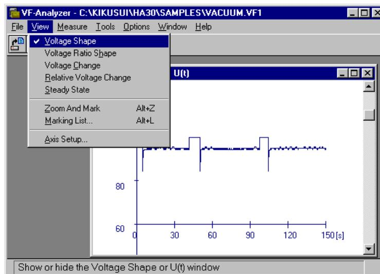
This window represents transition of voltage rms values for both positive and negative. Placing the mouse cursor on the graph screen, a set of data on the mouse cursor location will be displayed on the status line, which is in turn shown at the bottom of the application screen. Listed below are data contents shown on the status line:
