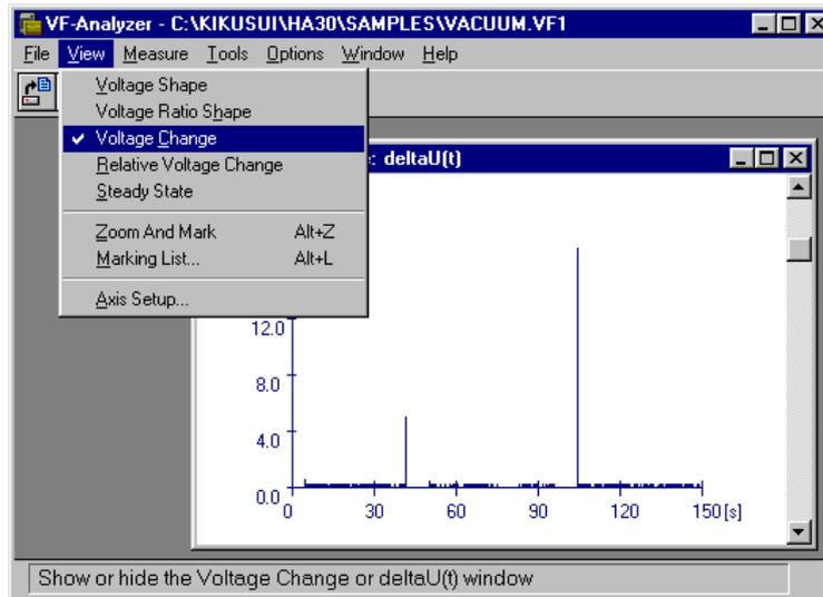
This window represents differences between adjoining data points of above mentioned **Voltage Shape** data as absolute values. Placing the mouse cursor on the graph screen, a set of data on the mouse cursor location will be displayed on the status line.
