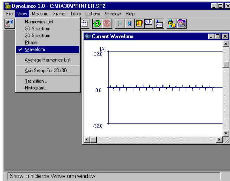
This window displays current waveform. The X axis indicates time, and the Y axis indicates current value (peak) respectively. This window is displayed as default, but you can show or hide it operating **View | Waveform** menu.
