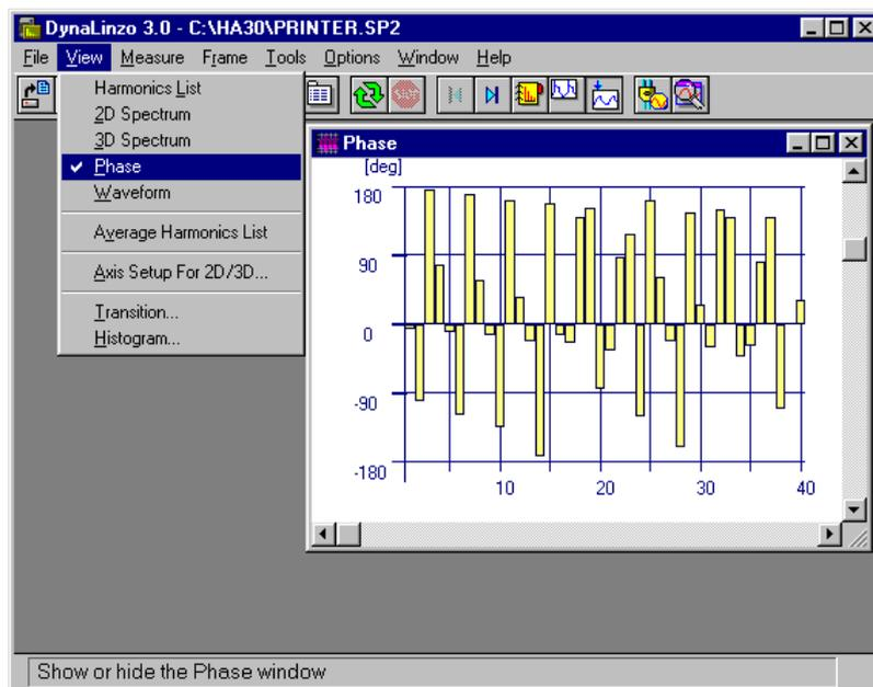
This window represents phase difference for each harmonics component referring to voltage phase of the PCR-L output. The X axis indicates the order of harmonics, and the Y axis indicates phase difference respectively. The unit is [deg], '+' means phase lead, and '-' means phase lag. This window is displayed as default, but you can show or hide it operating **View | Phase** menu.
