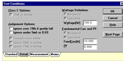
Sets items that are optional for a specific class. Depending on the class you have selected in above section, items corresponding the class will be automatically selectable. In addition, these settings can be changed even after measurement.
