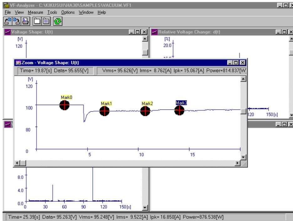
In this window, since markings must be done to get **Steady State** data, you should not mark groundless portions. Instead, you have to mark portions that voltages are stable and flat on the graph.
