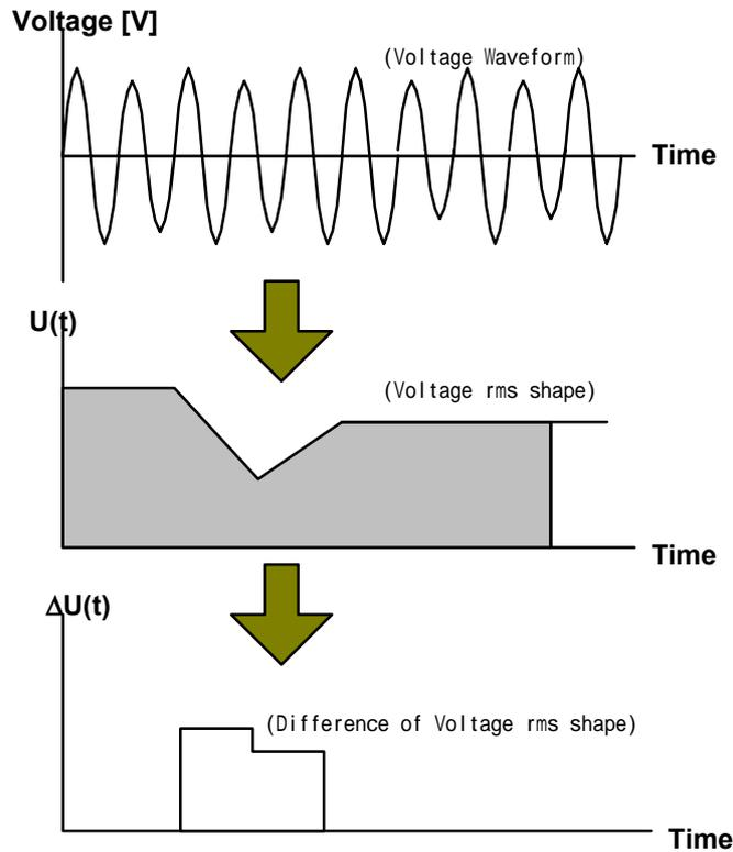
Furthermore,  $\Delta U_{max}$ ,  $d_{max}$ ,  $\Delta U_c$ , and  $d_c$  are to be calculated by the following rules:
