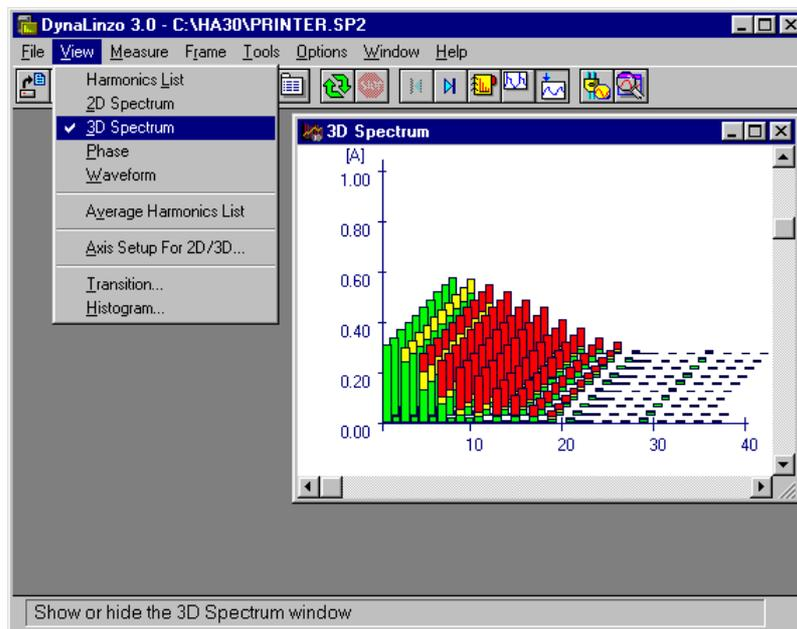
The 3D Spectrum is a multiple representation of the 2D Spectrum adding the time axis (Z axis). The most front column of the 3D spectrum chart designates the same data as that of the 2D and Harmonics List. Ten frames in total accompanied by time passage are also shown backward the most front data. In advance of time (or in advance of frame browsing), later data are coming from back to front on the screen.
