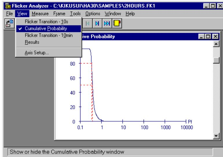
This window represents distribution status (cumulative probability) of PF values in a segment. This is not simply a histogram but a histogram that contains cumulated data. The X axis indicates PF values and Y axis shows frequency of corresponding data in a segment. In addition, the 50% and 80% marker lines are also displayed.
