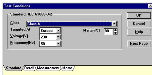
As fundamental settings for standard, basically you select judgement condition complying the IEC standard or the Japanese guideline. These settings can be changed even after the measurement.
